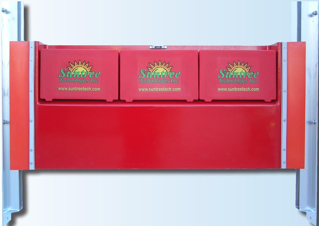
The optional SkimBoss® Floating Skimmer prevents floating solids and liquids from passing through the vault. Primary buoyancy is on the front inflow side which allows the skimmer to match fast rising water levels regardless of the level on the outflow side via patented Hydro-Variant Technology®. This then allows for maximum settling of sediments without compromising watershed hydrology.
